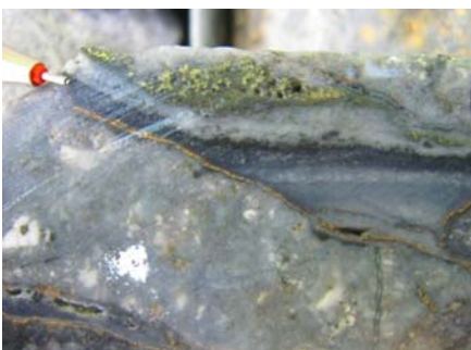
HUTDD027 160m: Colloform banded quartz-chalcopyrite-arsenopyrite-sphalerite veining
