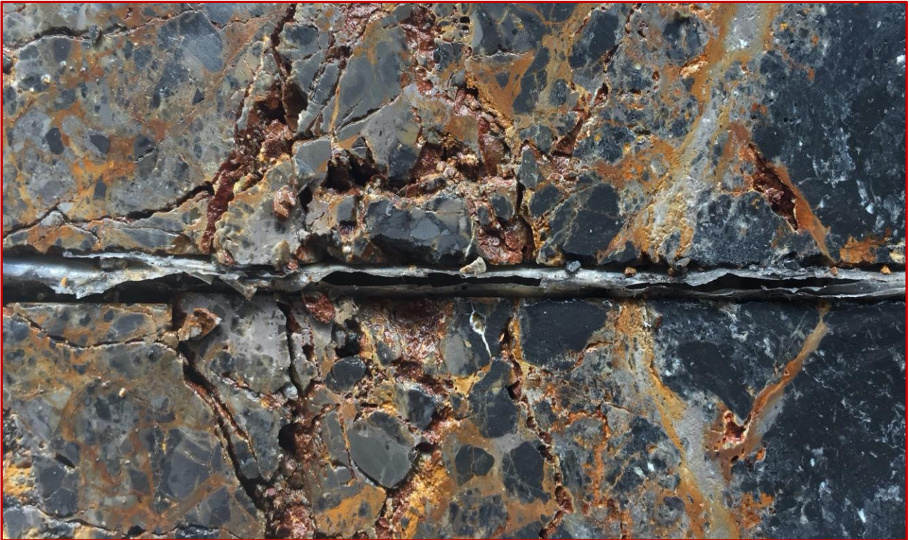
Photo 9 – SHDD606 at 147.2m down-hole: partly oxidised jasperoid breccia assaying 15.6 g/t Au
