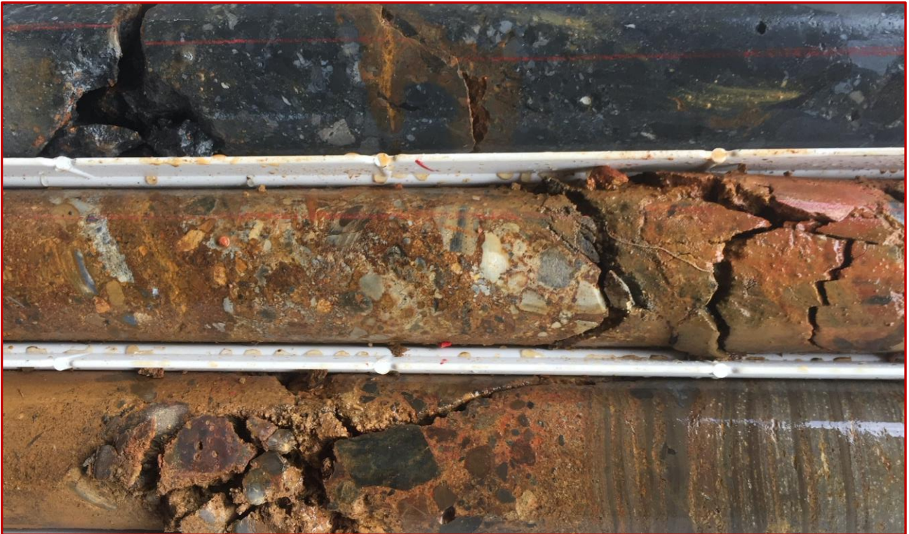
Photo 13 – SHDD609 at 129-131m down-hole: partly oxidised jasperoidal cave-fill sediments assaying 4-5 g/t Au
