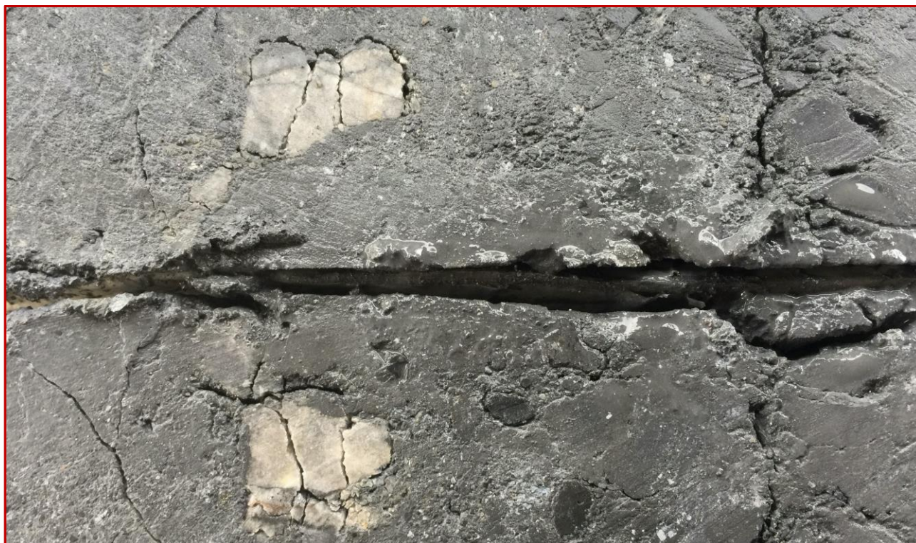
Photo 7 – SHDD606 at 158.3m down-hole: clay pyrite altered breccia assaying 11.2 g/t Au
