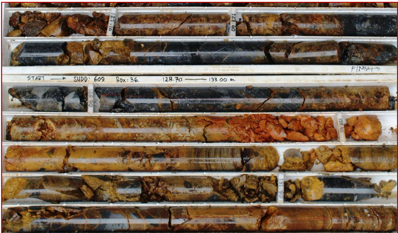
Photo 12 – SHDD609 at 127-133m down-hole: partly oxidised jasperoid breccia assaying 3.59-7.48 g/t Au
