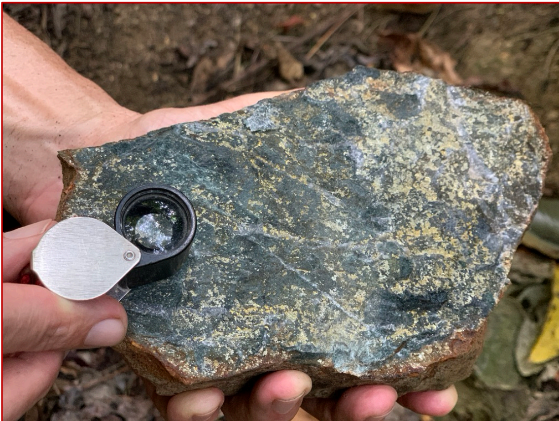
Figure 16 Sihayo-2 copper target – sample of freshly exposed of mineralised diorite featuring multi-directional quartz-magnetite and overprinting quartz-sulphide stockwork
