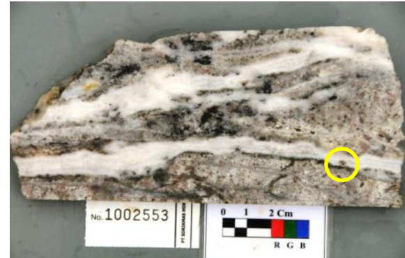
Weakly banded Colloform- Crustiform banded sheeted Quartz veins with visible gold (142 g/t Au)
