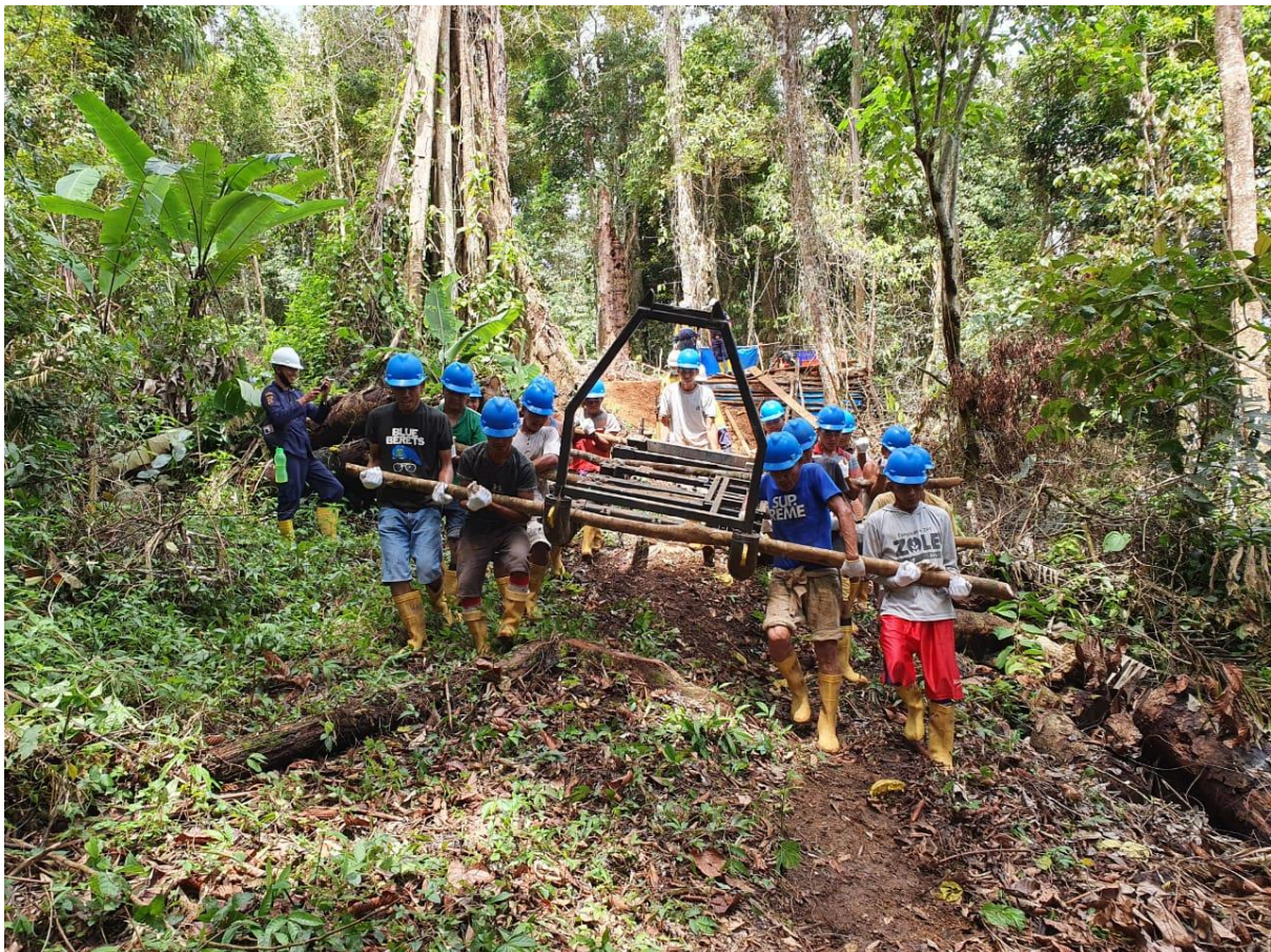
Photo 6: Sihayo-2 Prospect – Manual Rig Move
