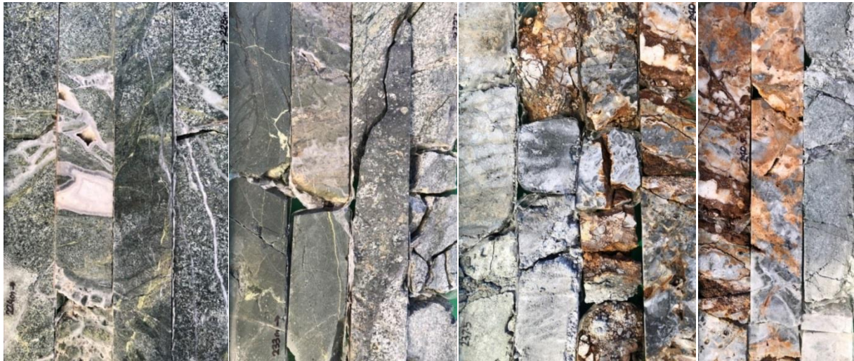
Figure 8: Penatapan - HUTDD090 - 209.0 - 248.0 m quartz stockwork and breccia vein averaging 0.26 g/t Au & 3.4 g/t Ag along the 39 m long core length
