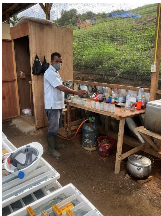
Tor Sigompul exploration core shed – ASD Terraspec analyses, bulk density & mag-susceptibility activities
