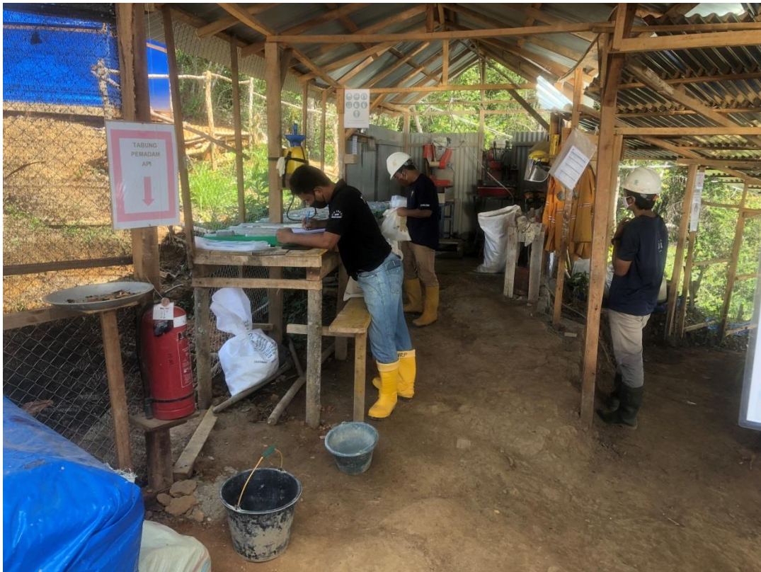
Tor Sigompul exploration core shed – Sroll core splitting & sampling
