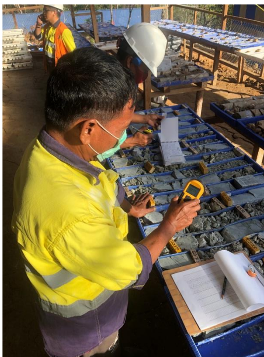
Tor Sigompul exploration core shed – ASD Terraspec analyses, bulk density & mag-susceptibility activities
