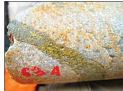
TTDD011 63.4m Quartz-pyrite-chalcopyrite veining in quartz-sericite-pyrite altered quartz diorite (62-64m: 3.04 g/t Au, 1310ppm Cu)
