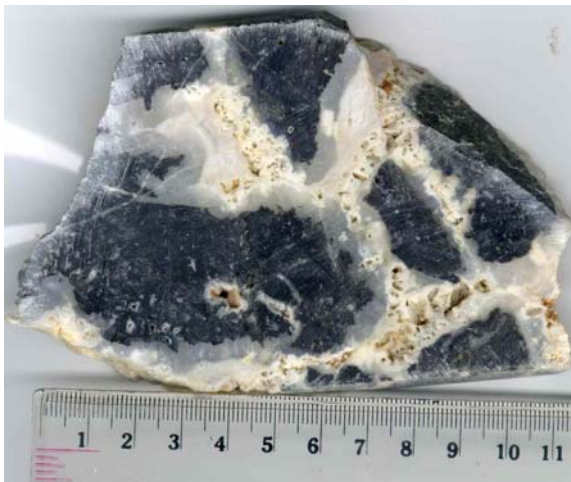
Fig. 5. Jasper cut by late colloform banded opaline-chalcedonic quartz +adularia from SAMDD002 (36.15m to 36.25m).
